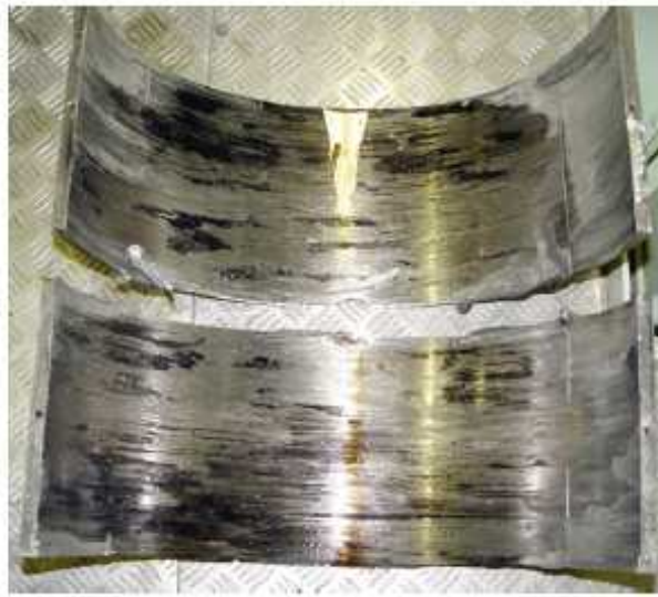
Pic. 1 Damage to cross-head bearing on a MAN 2-stroke engine
