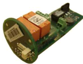
Pic. 5 The WIO200 main computer uses energy efficient components and only RoHs approved components.
